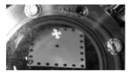
Maltese-cross shaped spot from an unfocused LaB<sub>6</sub> cathode seen on a custom phosphor screen inside the vacuum chamber
