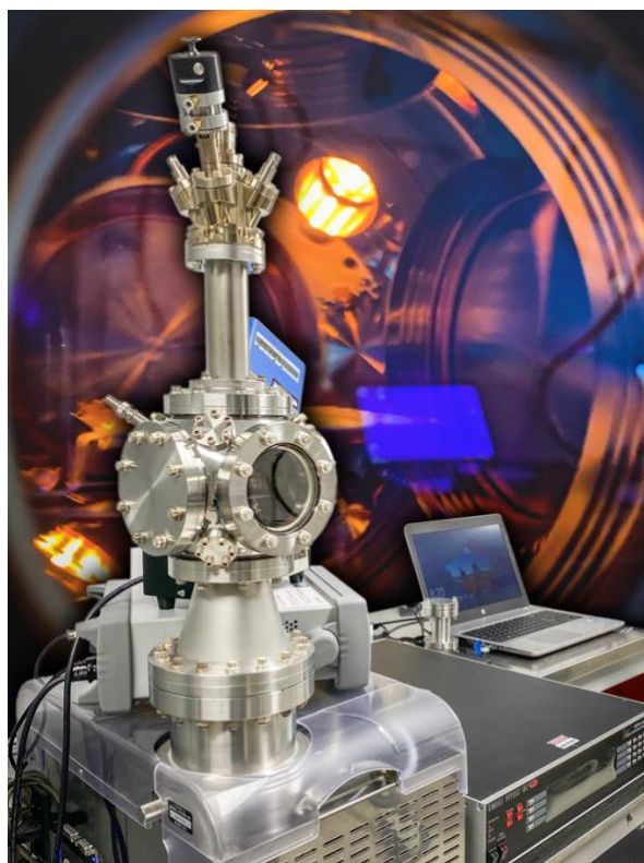
Upper Figure: Assembly, in progress, of an electron gun system. Lower Figure: Electron Gun System with electron gun, MCF vacuum chamber, vacuum pump, power supply, and laptop for Labview™ computer control interface. Image background is based on a typical view inside the chamber during operation.
